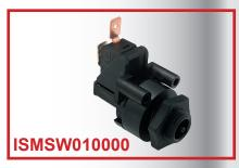
6A - 250 V micro-switch for pump. Held with a screw. Air connection: Ø mm. 3 Fixing hole: Ø mm. 14
