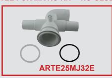
Special Tee-piece for the connection of the pump no glue with a deviation for the Microjet kit. Tee is installed directly onto the pump outlet with no glue. External dia. 25x25x32 mm. Microjet connection dia. 32 mm.
