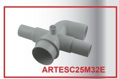
Special Tee-piece for the connection of the pump with a deviation for the Microjet kit, installation with glue. External dia: 25x40x25. Microjet kit External dia:: 32 mm
